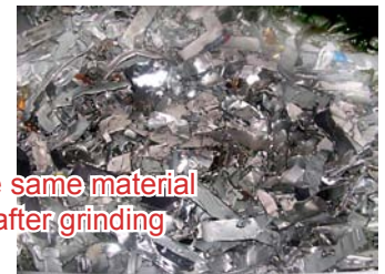
after crushing, sorting is facilitated
