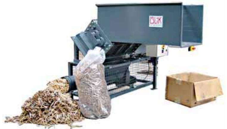
BLiK B400 crusher, non stop screw output and bag for destroying cardboard packaging without flattening. Excellent for making packaging sheets.
