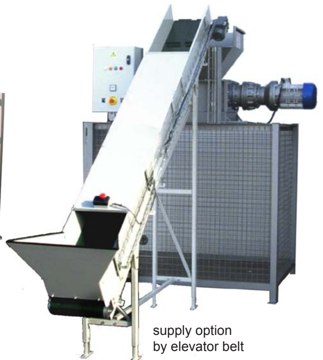
BLiK B400 crusher, non stop screw output and bag for destroying cardboard packaging without flattening. Excellent for making packaging sheets.
