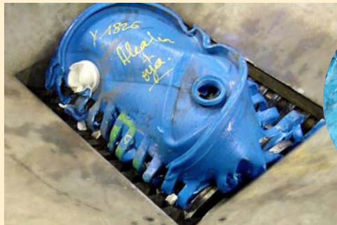
Crushing plastic containers in a BLiK B600.
