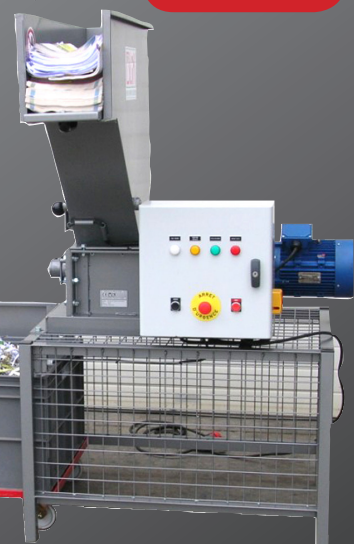
BB230 with output «BLIK endless screw» filling bag upright
