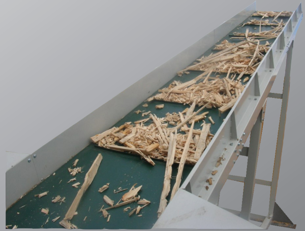
Wood evacuation after separation of the metallic points.
