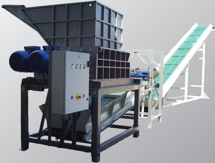
B840-1250 with evacuation conveyor and magnetic sorting by overband in order to crush pallets
