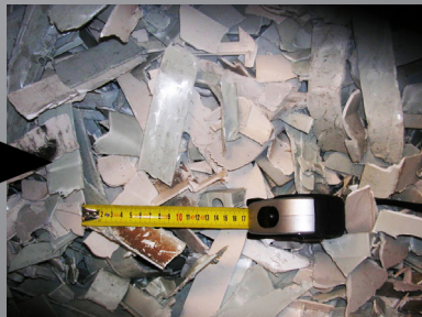
After magnetic sorting by overband : the plastic
