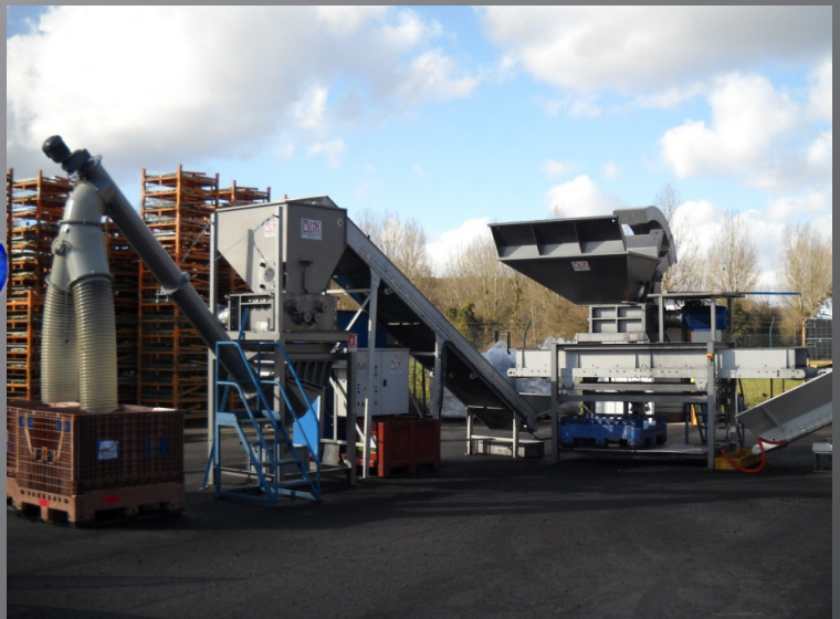
BLIK B600 Crusher : destruction of plastic containers: the only way to reduce their volume because if they are simply pressed, they gradually bounce back into shape.
