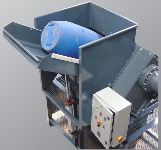
BLIK B600 Crusher : destruction of plastic containers: the only way to reduce their volume because if they are simply pressed, they gradually bounce back into shape.
