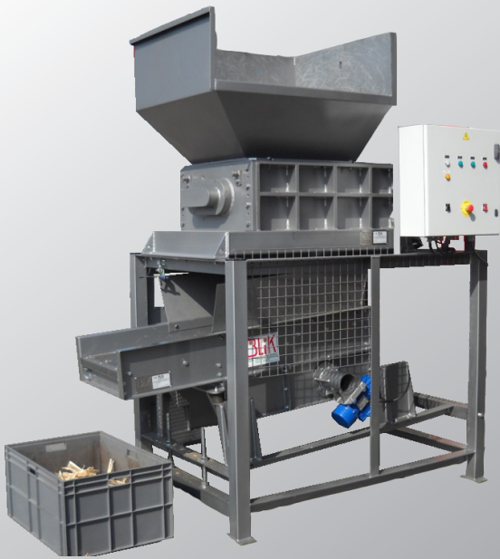
BLIK B600-750 crusher evacuation of vibrating screen for separation
