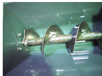
Evacuation via screw on the back in a dedicated compartment.
